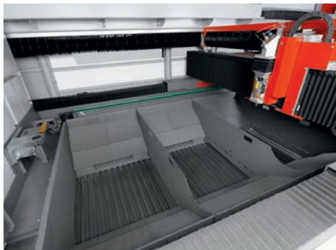
WAVE-BELT dopravník v stroji. WAVE-BELT conveyor within the machine.
