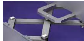
5 Synchronising device (harnesses) for fast-running telescopic covers
