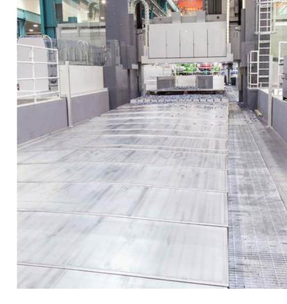
covers must also be able to cope with these challenges. This is where telescopic covers with harness mechanisms are used. So-called differential drives serve to synchronize the boxes and eliminate impact pulses.
