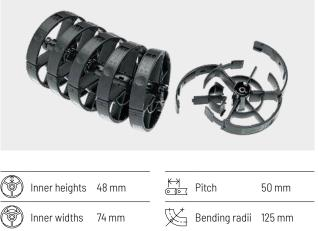
The basic construction is similar to the ROBOTRAX® types with single part design. Swiveling crossbars with snap locks make it easy to open and safely close the cable carrier. In addition, the three chambers can be divided horizontally and vertically by a divider module for precisely separating cables and hoses.
