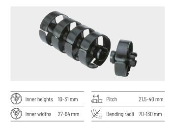
The basic structure of ROBOTRAX<sup>®</sup> consists of plastic links. These have spherical snap-on connections on both sides. This allows the individual links to be snapped together to form a cable carrier. Protectors ensure that the bending radius does not fall below the minimum in any direction. The links can be rotated in the radial direction (see table values). The cables can be separated in three chambers.
