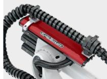
With fast movement sequences and large work envelopes, the relatively long carriers knock against the robot arm. The repeated impact significantly reduces the service life of the cable carrier and the cables within, and the entire system can fail. Downtimes cause high costs and problems in the manufacturing process - so they have to be avoided.
