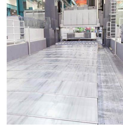
covers must also be able to cope with these challenges. This is where telescopic covers with harness mechanisms are used. So-called differential drives serve to synchronize the boxes and eliminate impact pulses.
