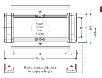
The maximum cable diameter strongly depends on the bending radius and the desired cable type.
