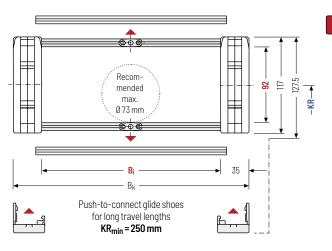
The maximum cable diameter strongly depends on the bending radius and the desired cable type.
