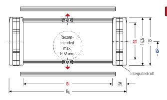
The maximum cable diameter strongly depends on the bending radius and the desired cable type.
