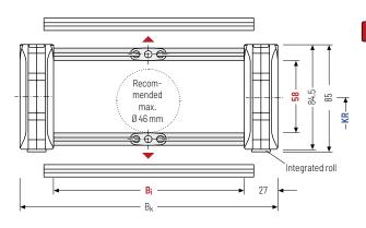
The maximum cable diameter strongly depends on the bending radius and the desired cable type.
