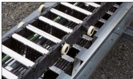
TRAXLINE long travel testing at TSUBAKI KABELSCHLEPP headquarter
