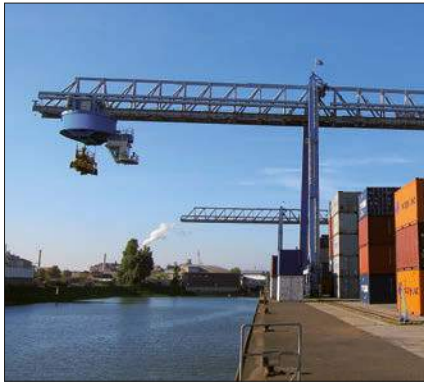
TRAXLINE in long travel crane applications
